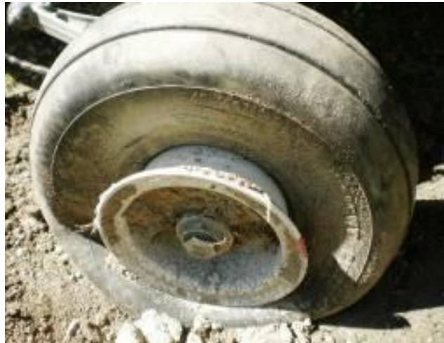
RH- Main wheel deflated and damaged
