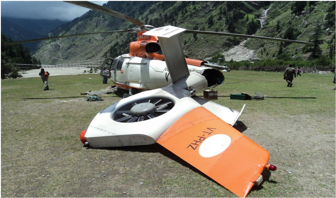
Aft structure of helicopter VT-PHZ was substantially damaged
