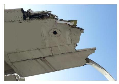
Wing tip and wing tip fence area sheared off and found in drain.
