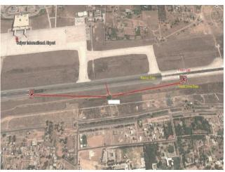
The decision of PIC to disengage the autopilot was the last inappropriate act which caused the aircraft to deviate to left from localiser resulting in the aircraft landing (with both landing gears) on the soft ground.
