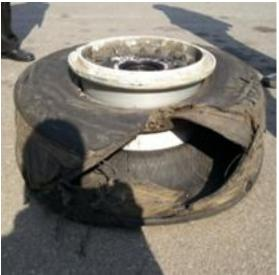
The aircraft had touched on the left side of the runway on soft ground. There was no damage to the aircraft on its first impact with the soft ground. The aircraft had rolled and then the left wheel had gone over the drain boundary area. The left main wheels got de-capped / damaged during this roll over/ skidding and during final stoppage with application of brakes.
