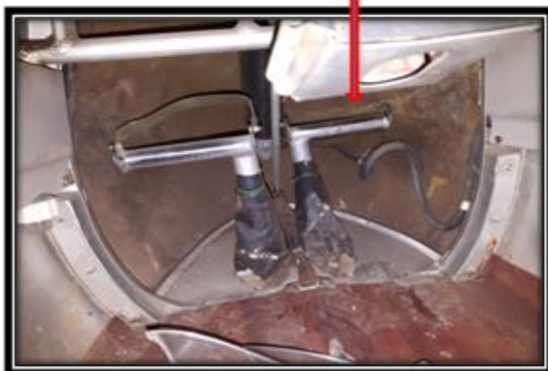
Right side Rudder Pedal damaged
