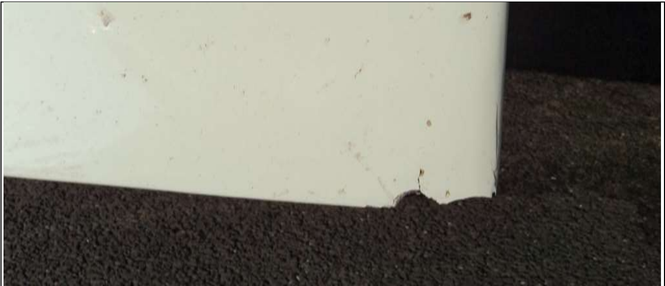
Damage observed on inner edge of the LH flap
