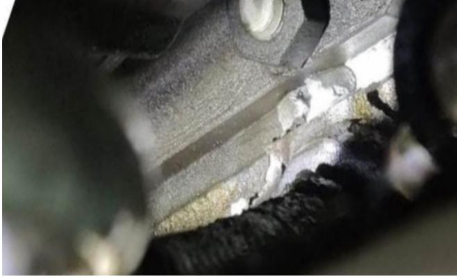
The only damage observed externally was an oval fracture at the bottom of cylinder No 04 through which there was oil leakage.
