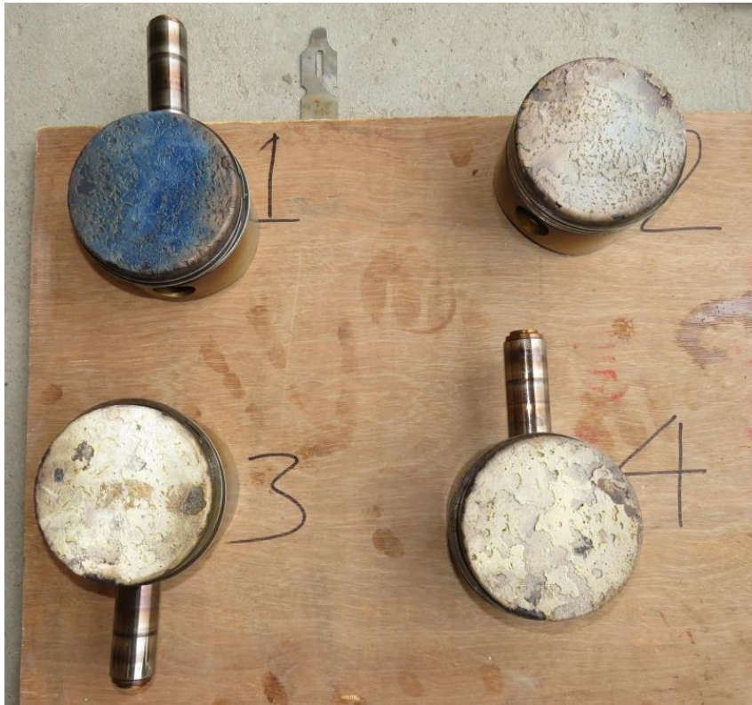
Fig 15: Blue Colour deposit and Lead deposit on the pistons
