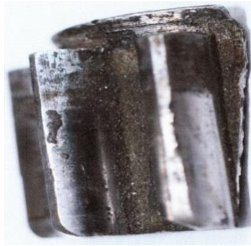
Fig 20: Pitting on the gear
