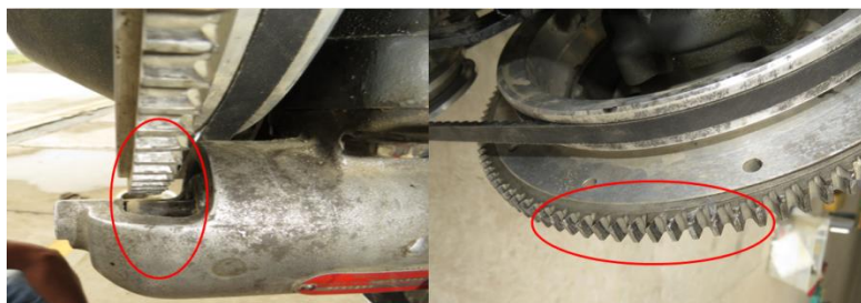
Fig 11: Broken Starter Gear and Ring Gear teeth
