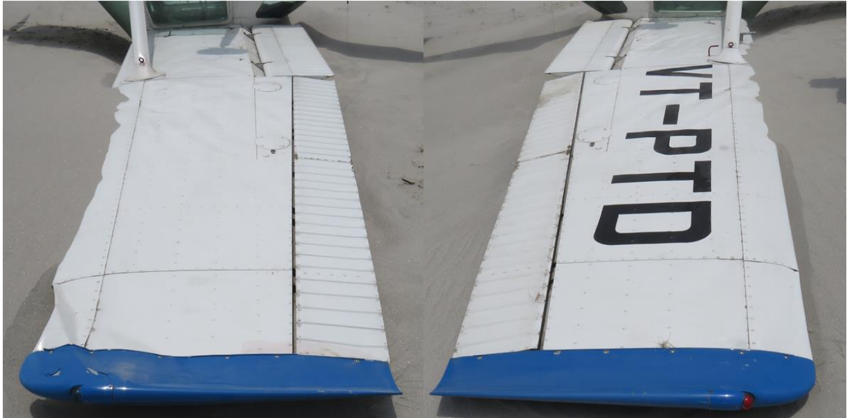
Fig 4: Damages to LH and RH wing
