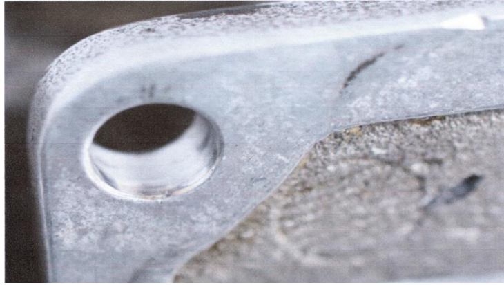
Fig 19: Rubbing marks on mounting holes
