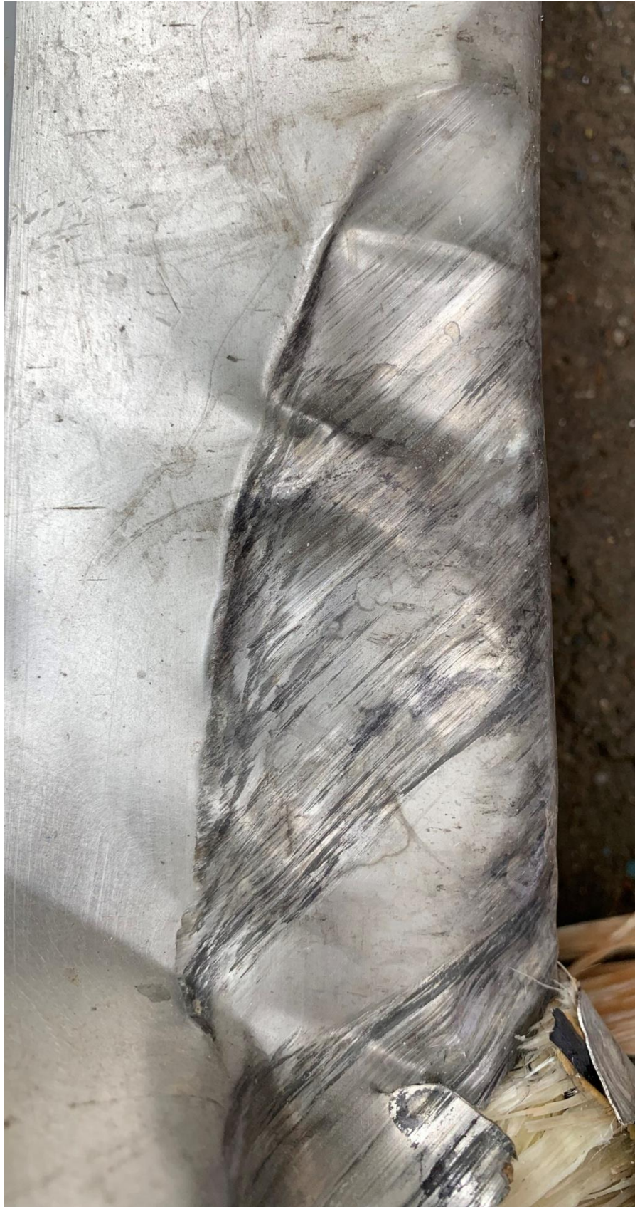
Rubbing marks of trolley cable on LE of main rotor blades
