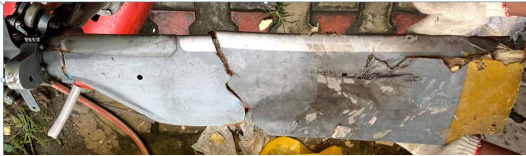
Sheared off tail rotor blade
