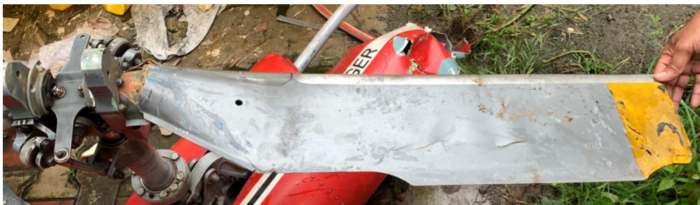
A tail rotor blade in full with consequential impact damages
