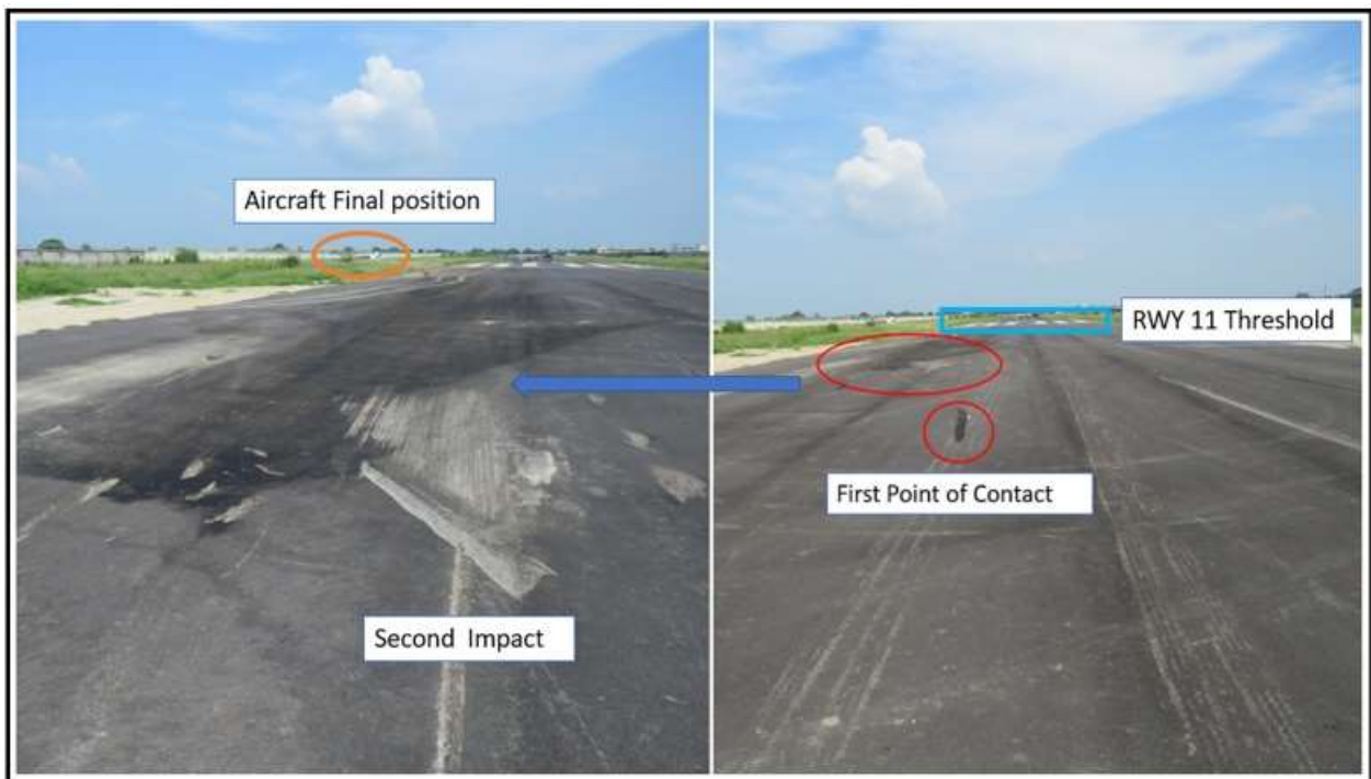
Fig-8: Landing Gear Tyre Markings on Runway
