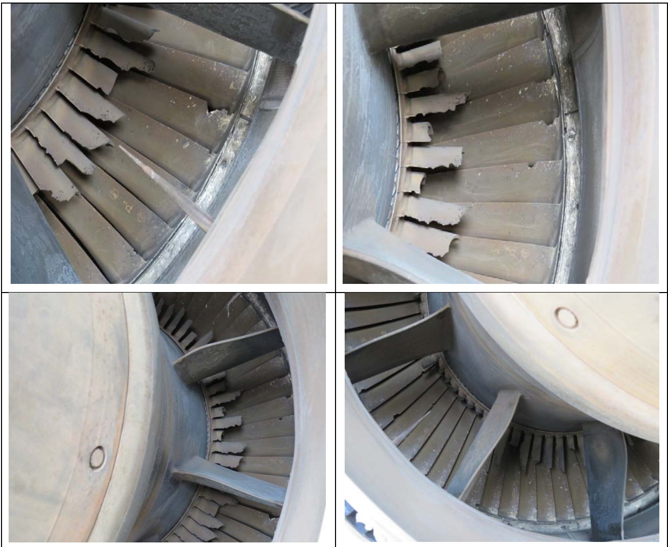
Figure 1: Engine LPT 3rd Stage blades were found damaged during inspection.
