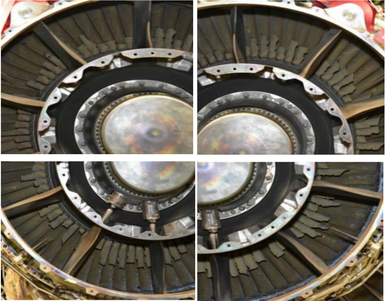
Figure 1: Engine LPT 3rd Stage blades were found damaged.
