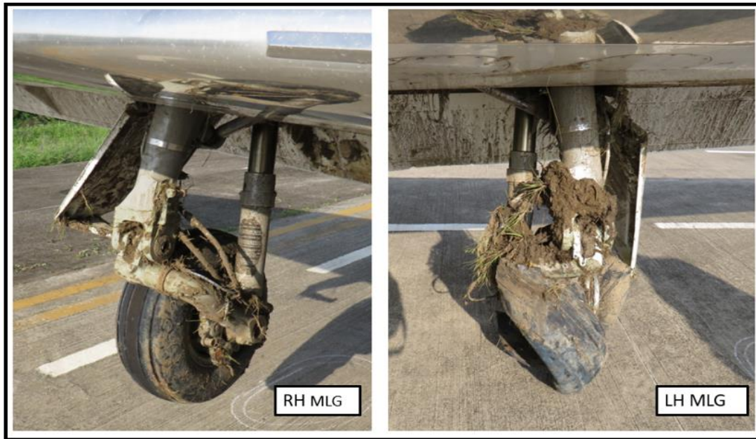
Fig 5: Front view of damaged MLG
