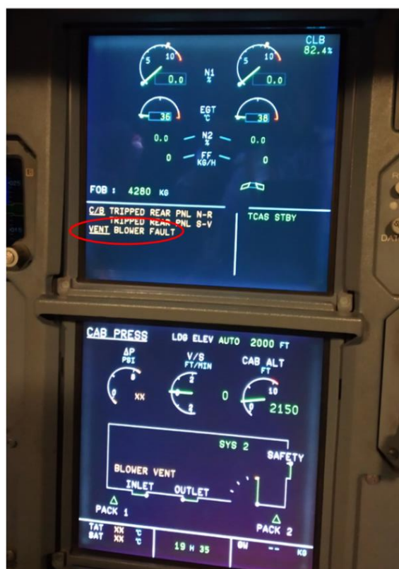
Fig. 6: Vent Blower Fault
