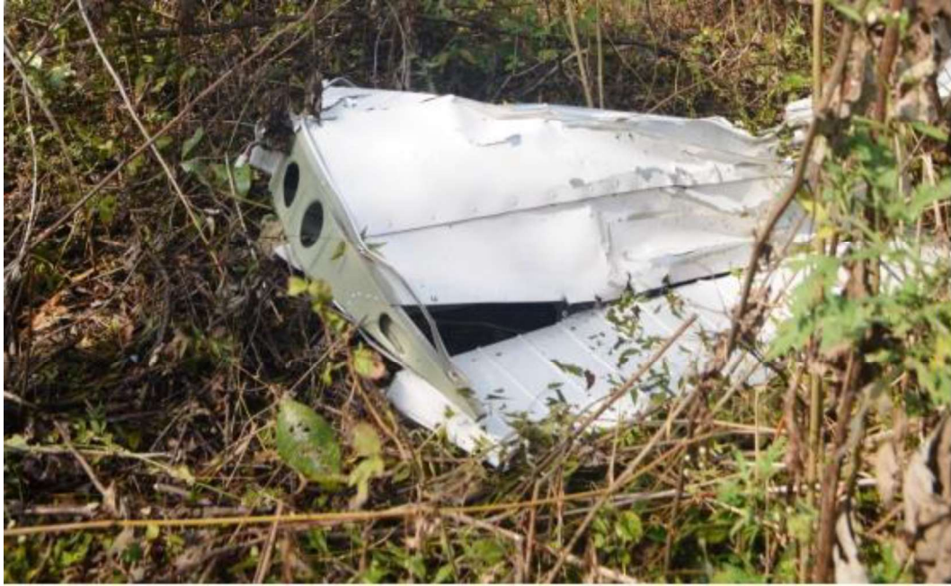
Figure 8 : LH Wing portion separated due impact with the trees
