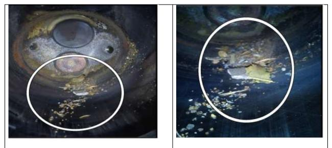
Pebbles, broken piece of oil sump, a piece of dry leaf of tree and dust were found inside the combustion chamber indicates that the engine was running at the time of impact.
