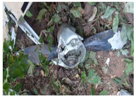
Sudden impact of propeller shows breaking of shaft under power
