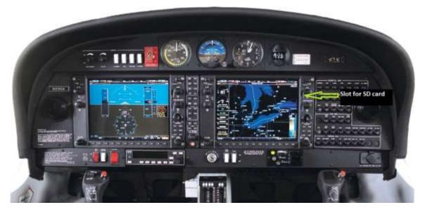
Location of Secure Digital (SD) card which records aircraft primary parameters
