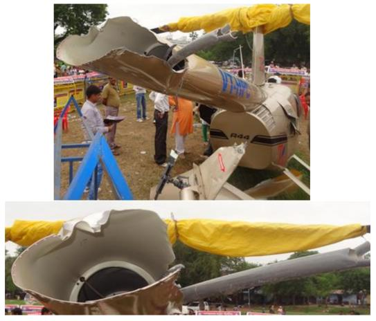
Photographs showing separation of tail rotor boom from the rivets
