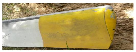
Photographs showing exposed bond line on the blade (without debonding)
