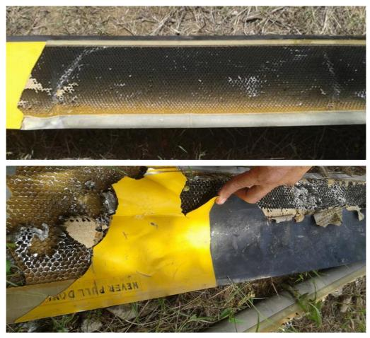
Photographs showing peeling of the blade skin with consequentinal damage to honey comb structure
