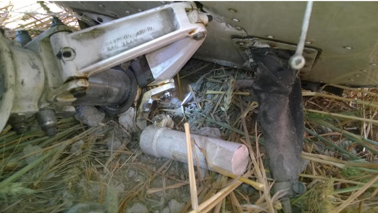
**DAMAGE TO NOSE LANDING GEAR**
