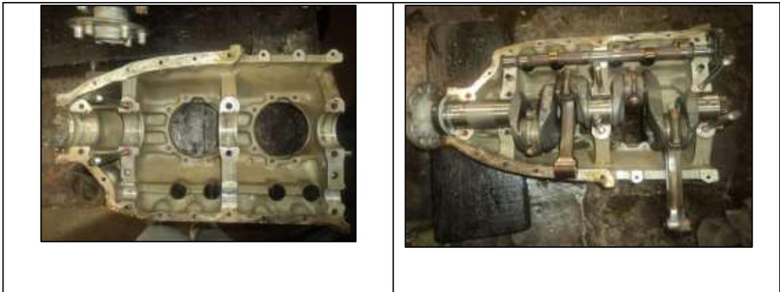
*The condition of Crankcase, Crankshaft, Camshaft & Connecting Rods were found satisfactory.*
