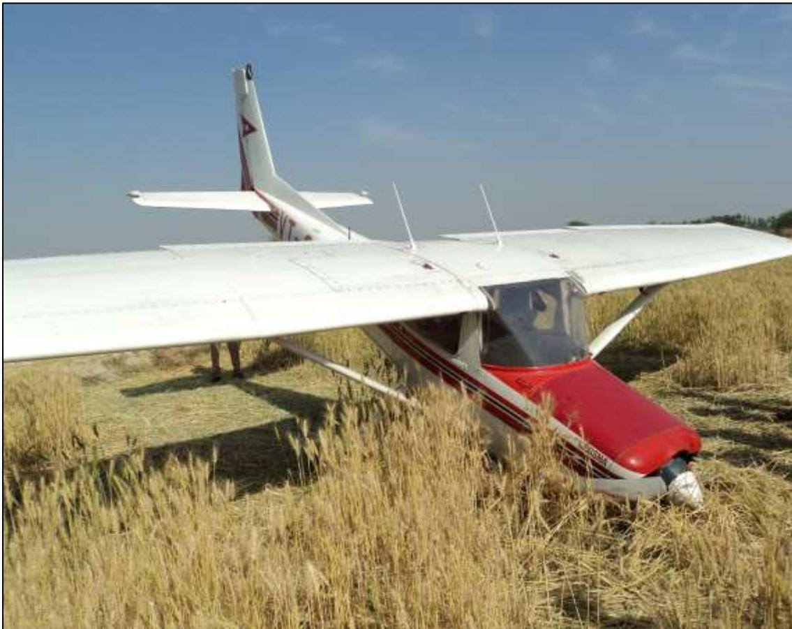
**Final rest position of the aircraft in Nose Down condition.**
