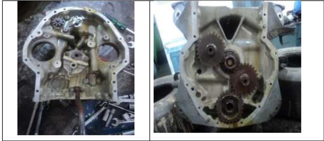
*The condition of Oil Pump and housing, Tachometer drive, Vacuum pump drive, Crankshaft gear, Camshaft Gear and Magnetos drive gears were found intact. No damage observed.*
