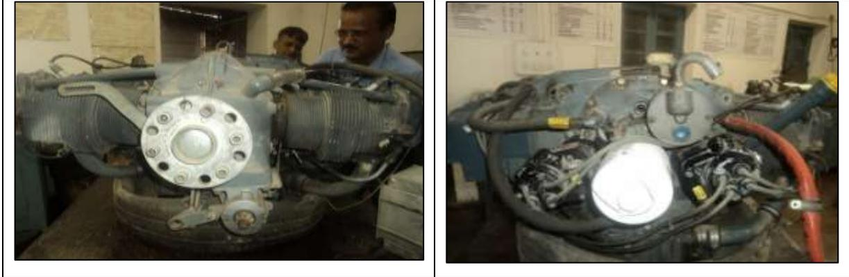
*The engine was found Intact and no external damage observed. All the accessories were found installed and intact except the carburetor.*
