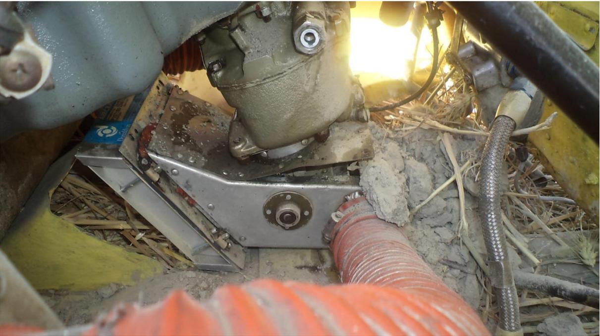
DAMAGES TO ENGINE & ENGINE MOUNT
