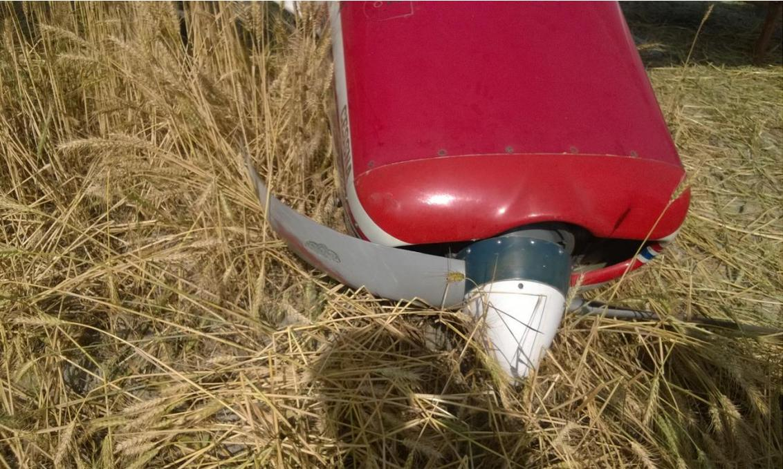
**DAMAGE TO PROPELLER**
