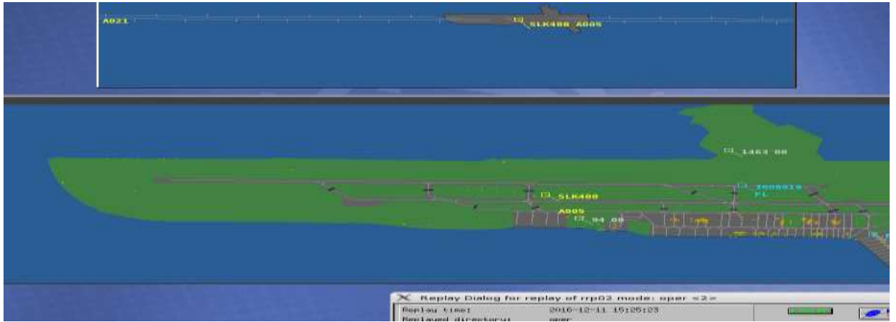
Figure 11: At time 15:25:23, SLK488 going around, passing 500 feet, offset to right, position abeam Twy B whereas IGO6619 airborne, position abeam Twy C
