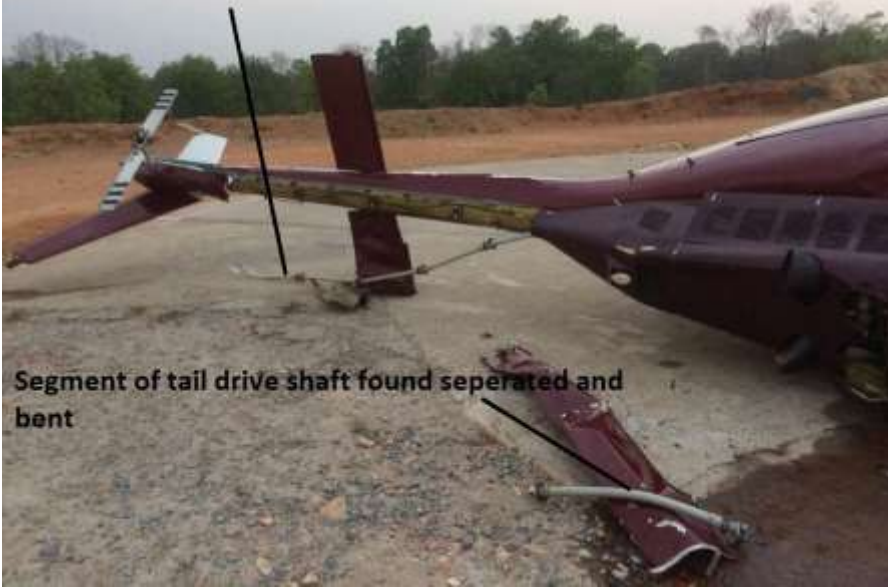
Tail Drive Shaft found broken and seperated from the tail boom
