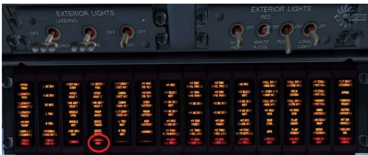
Touched runway light in overhead warning light panel in cockpit
