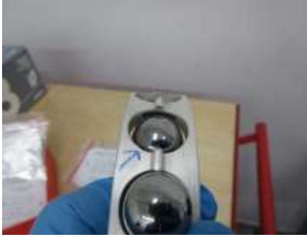
No. 1 Brg. - Flaking at cage
