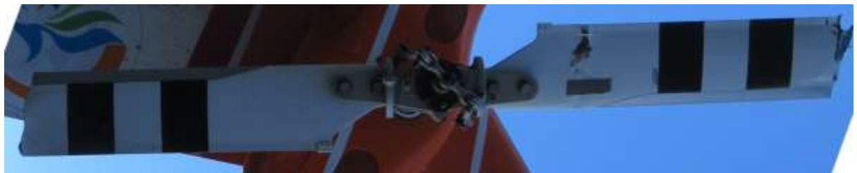
Both tail rotor blades sheared off identically at about 150 mm from tip of the blade.
