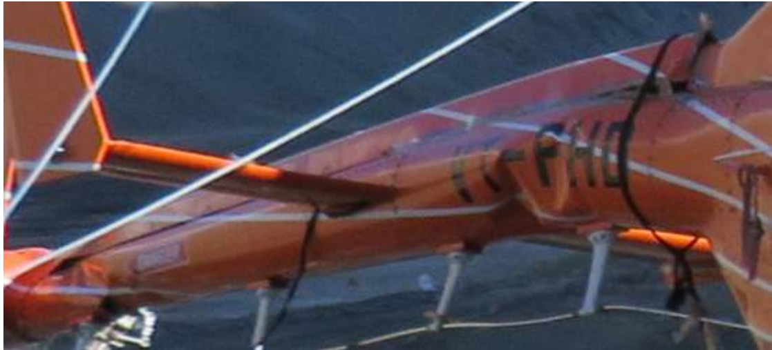
Tail boom dented and cracked at two places. Tail boom buckled downwards from the tail boom joint.
