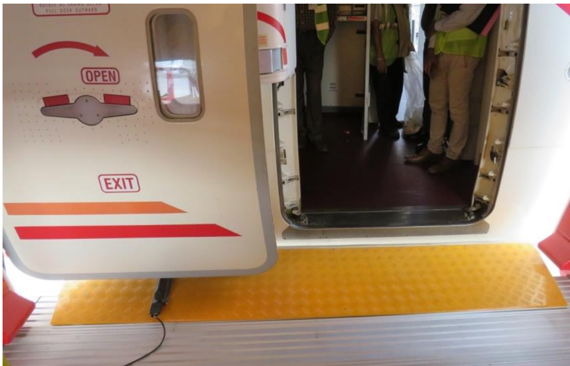
Fig. 5: Step Ladder with movable platform aligned to the aircraft
