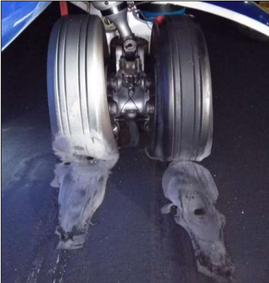
DAMAGE TO STARBOARD MAIN WHEEL ASSEMBLY
