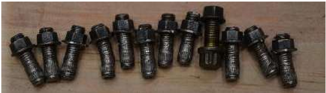
Fig-15: Damaged IGB studs
