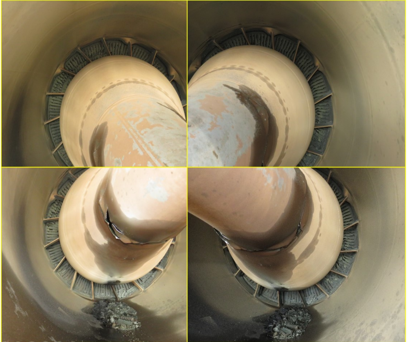
Fig-2: Damaged Centerbody - Close View (viewed from rear)
