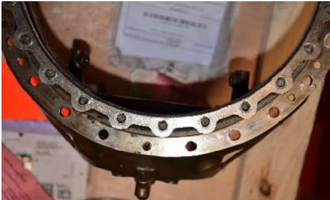
Fig-14: IGB Broken Studs
