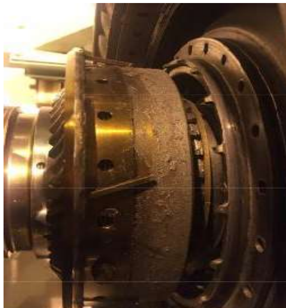
Fig-17: Damaged No 3B Bearing Finger Housing
