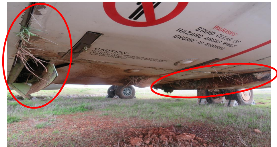
Pic 2: Damaged LH Engine Cowl.
