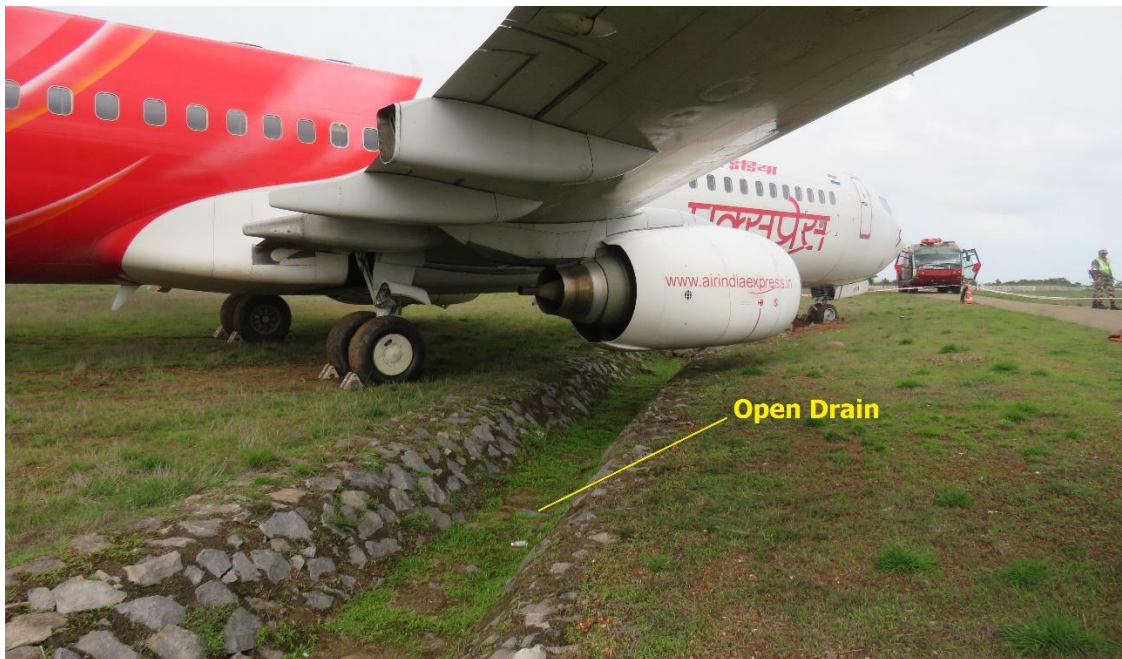
Pic 10: Aircraft stopped after Nose wheel ran over open drain.
