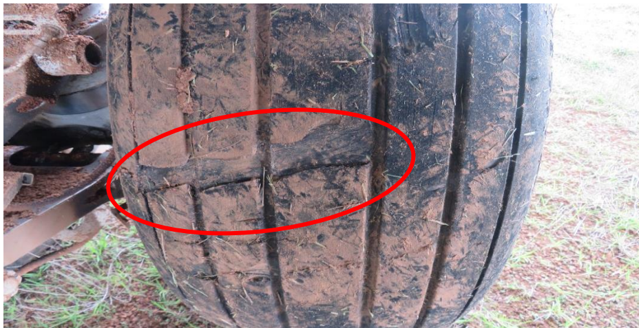
Pic 3: Cut marks on MLG tyre.
