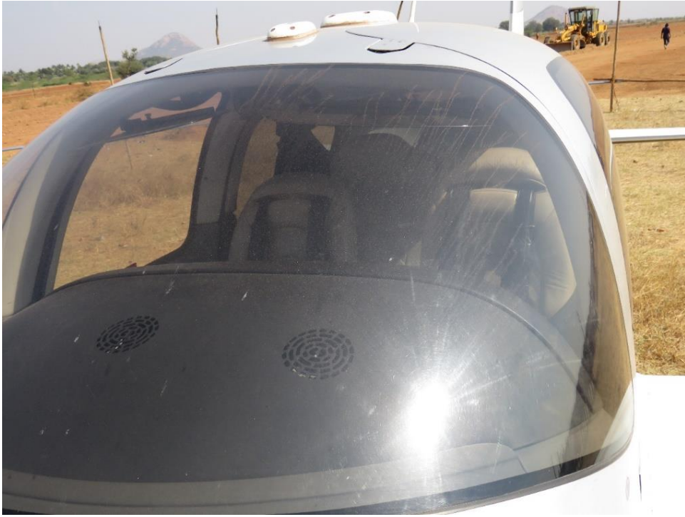
Fig 6: Fuel streaks on Aircraft Windshield
