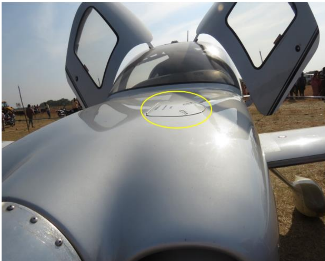
Fig 7: Oil Inspection Panel on Engine Top Cowling
