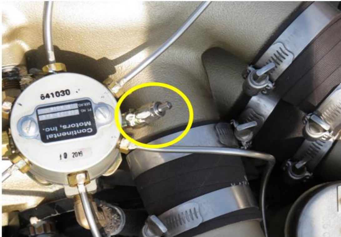
Fig 4: Blanking Nut Position on Fuel Flow Divider Unit
