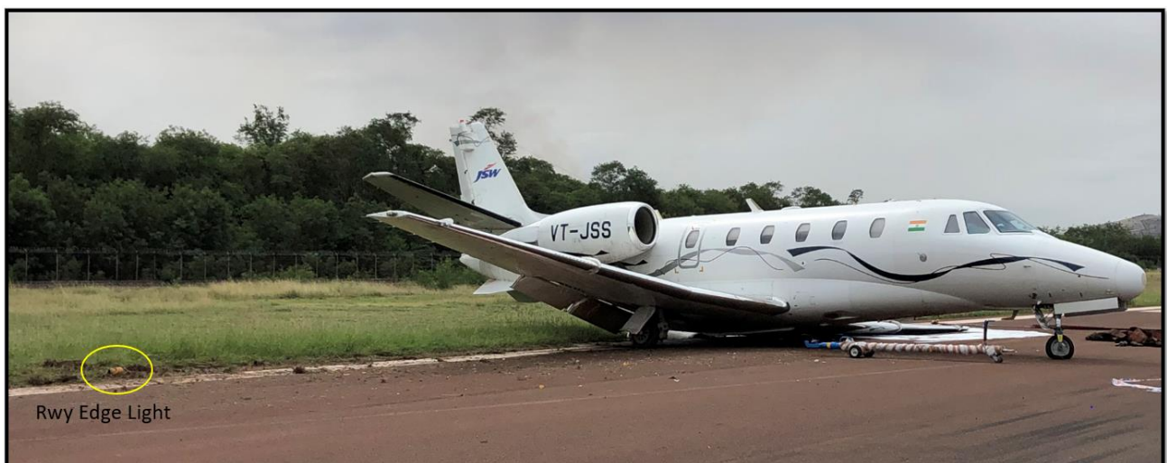
Fig 1: Broken runway edge light
