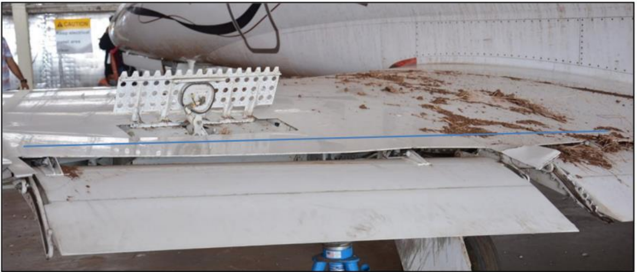
Fig 18: LH upper wing skin bent in flap area (blue line for reference)
