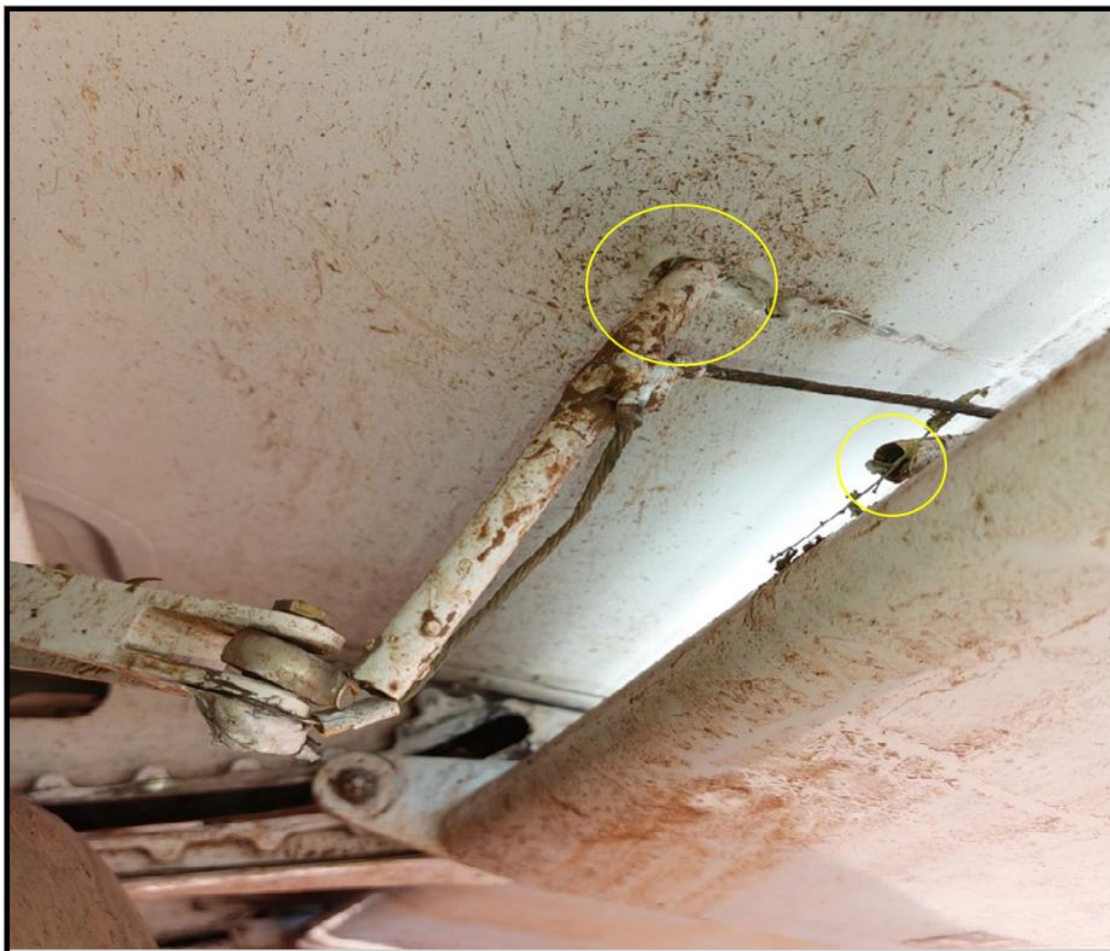
Fig 16: Flap Bell crank & Pushrod
