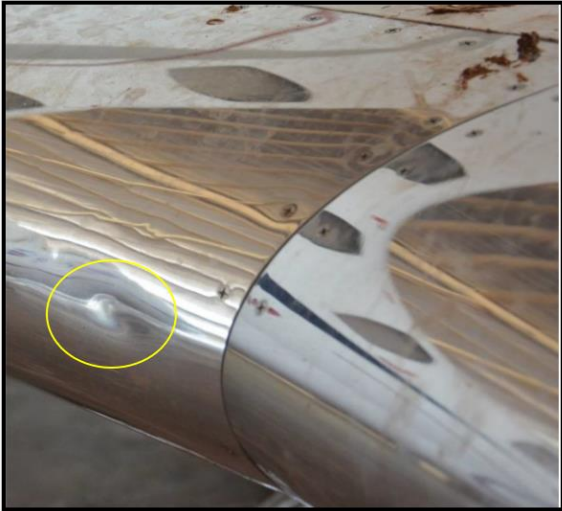
Fig 20: Dent on leading Edge
