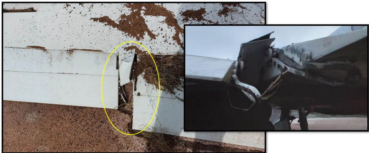
Fig 15: Damages on LH Flap
