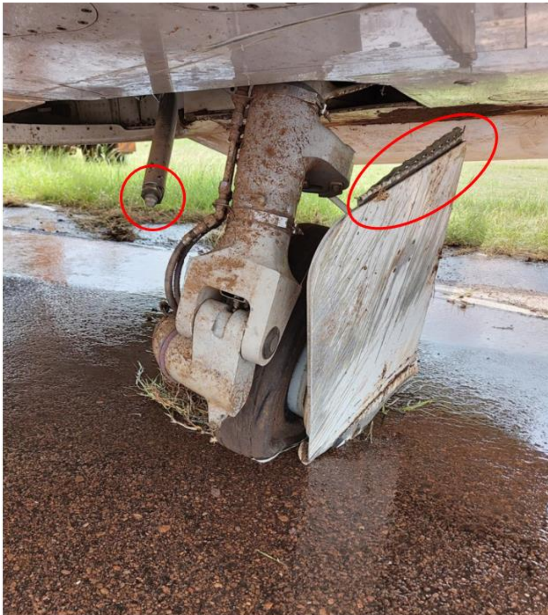
Fig 25: Detached Landing Gear Door (LH) and broken Actuator rod
