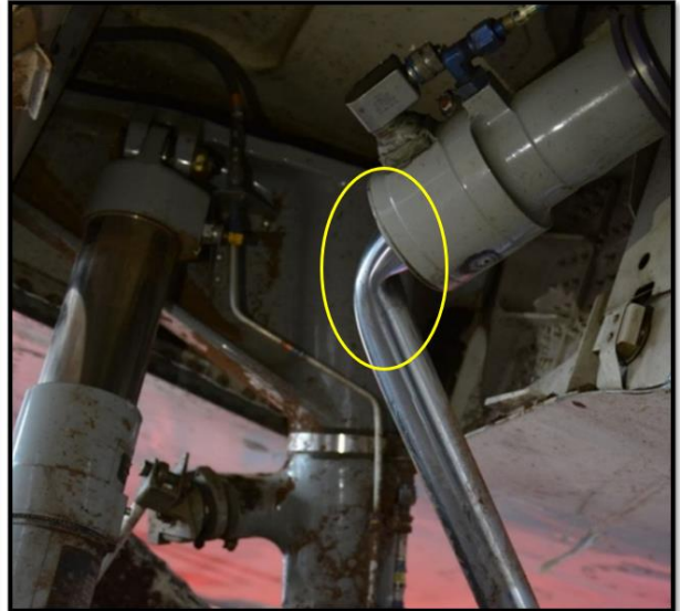
Fig 24: Piston Rod bent
