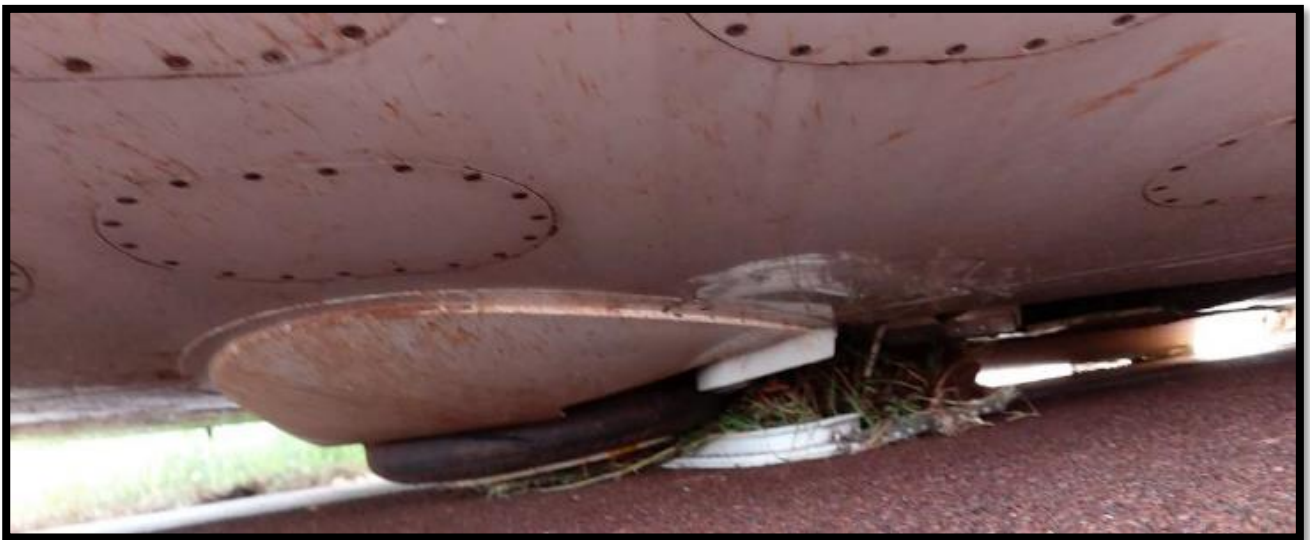
Fig 22: Collapsed LH MLG
