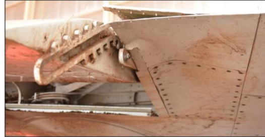
Fig 12: Skin separation on LH wing
