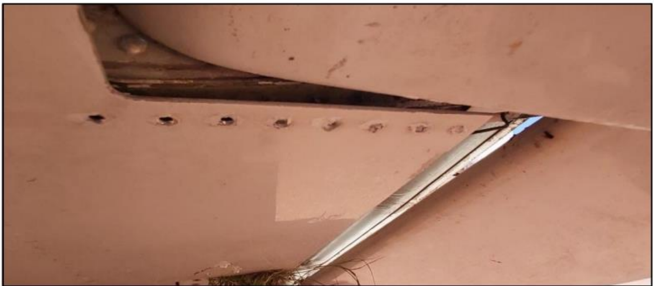
Fig 13: Holes on lower surface
