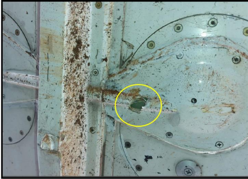
Fig 29: Damage on Keel Beam Area
