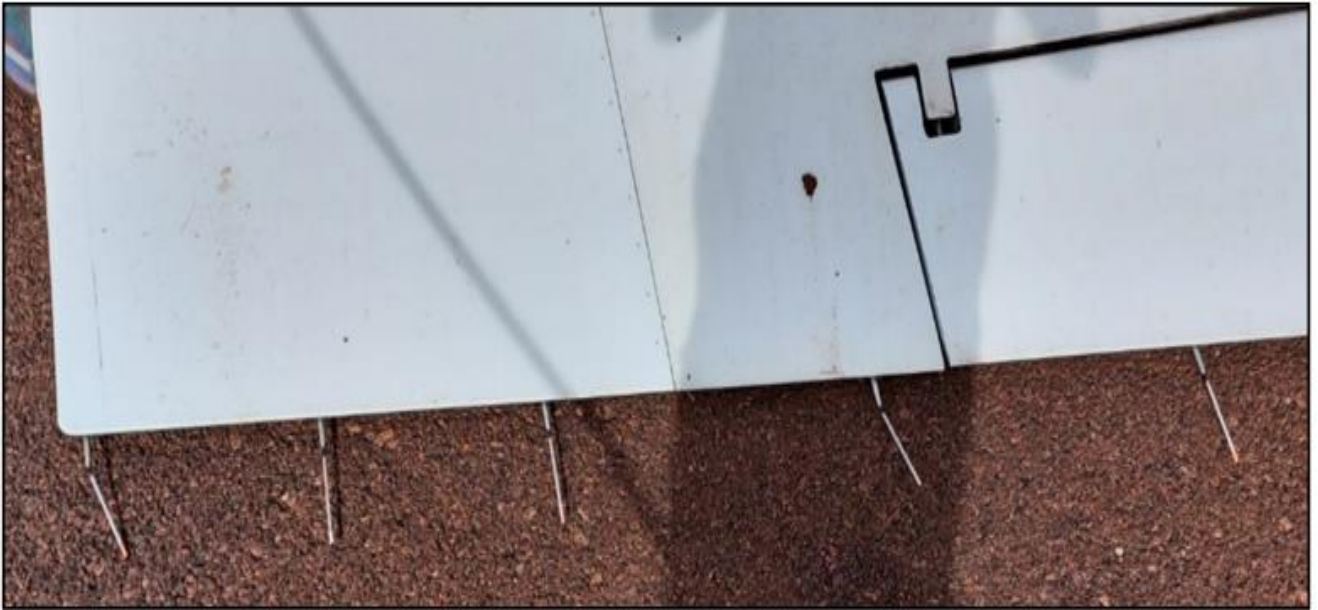
Fig14: Damaged Static Wicks
