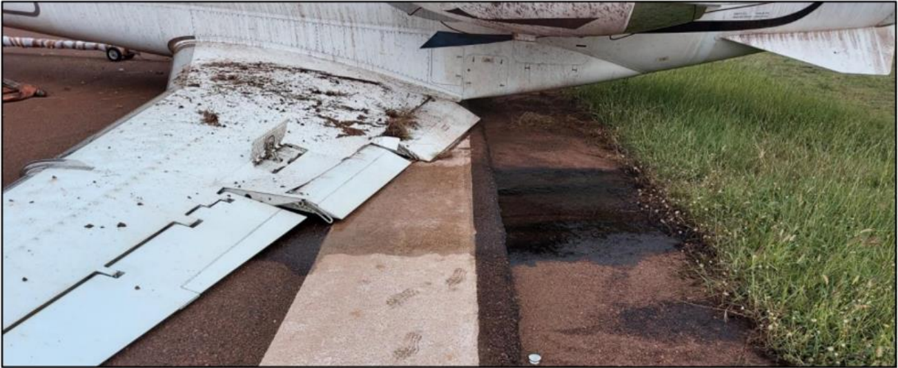
Fig 31: Fuel leaked from left Wing Tank
