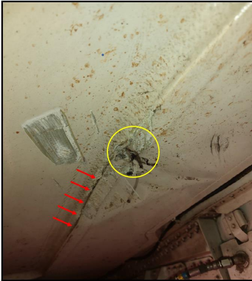
Fig 26: Hole and crack on Wheel Well upper surface
