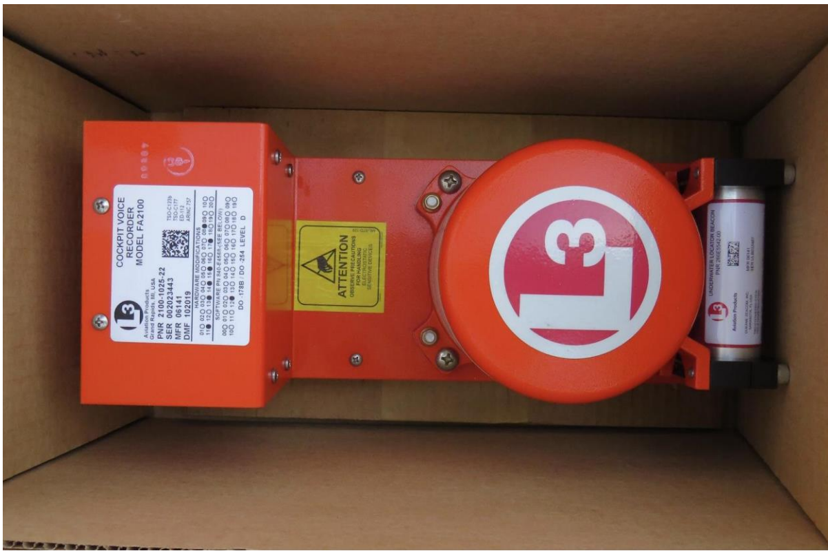
Fig 14: Photograph of actual recovered CVR
