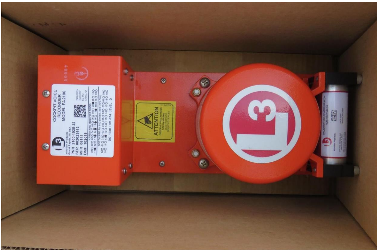
Fig 14: Photograph of actual recovered CVR
