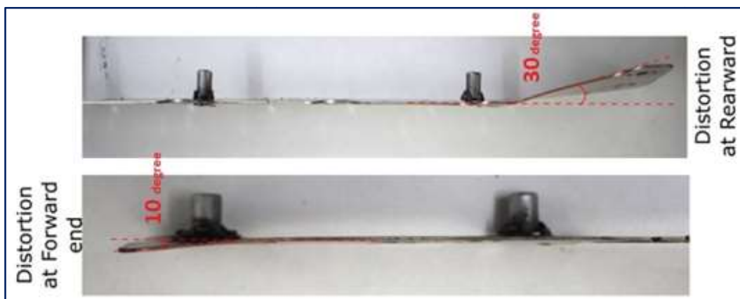
Fig 28: Top metal strap bend
