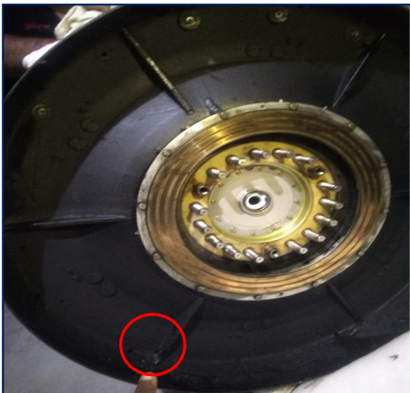
Fig12: Back plate hub assembly damages
