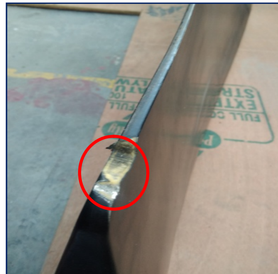
Fig13: Damages in the propeller blade
