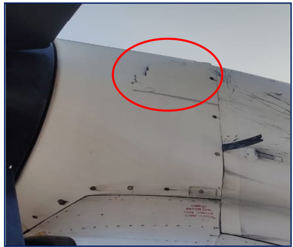
Fig 9: Cracked inboard upper forward cowling
