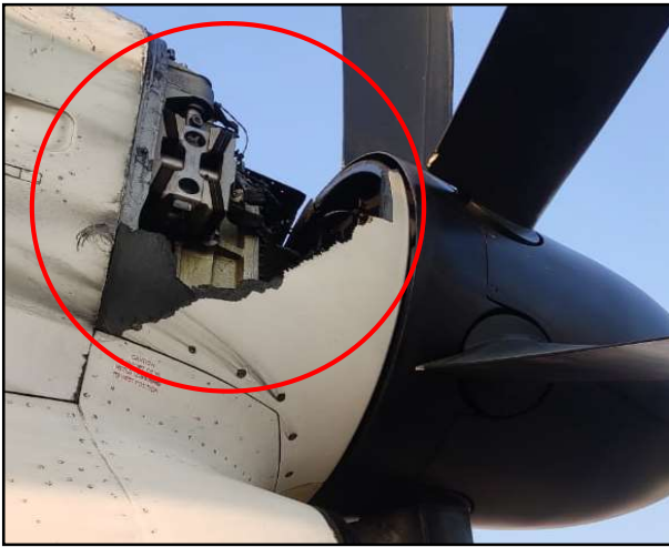
Fig 8: Missing outboard upper forward cowling
