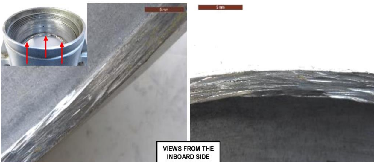
Figure 35 – Details of some nicks visible on the side surface of the shoulder of the support bearing sleeve assembly mating with the inboard bearing (red arrows), due to the contact with the relief elements of the inboard locking nut.
