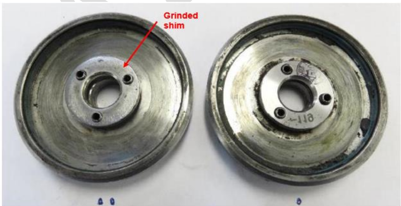
Figure 7 – Details of the shims installed under the two hub flange assemblies (Fig. 6). The one under the hub flange with the washer foreseen in the maintenance manual is evidently grinded.
