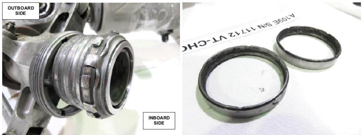
Figure 38 – Details of the duplex bearing as arrived in the laboratory. The outer rings were separated from the inner ones.
