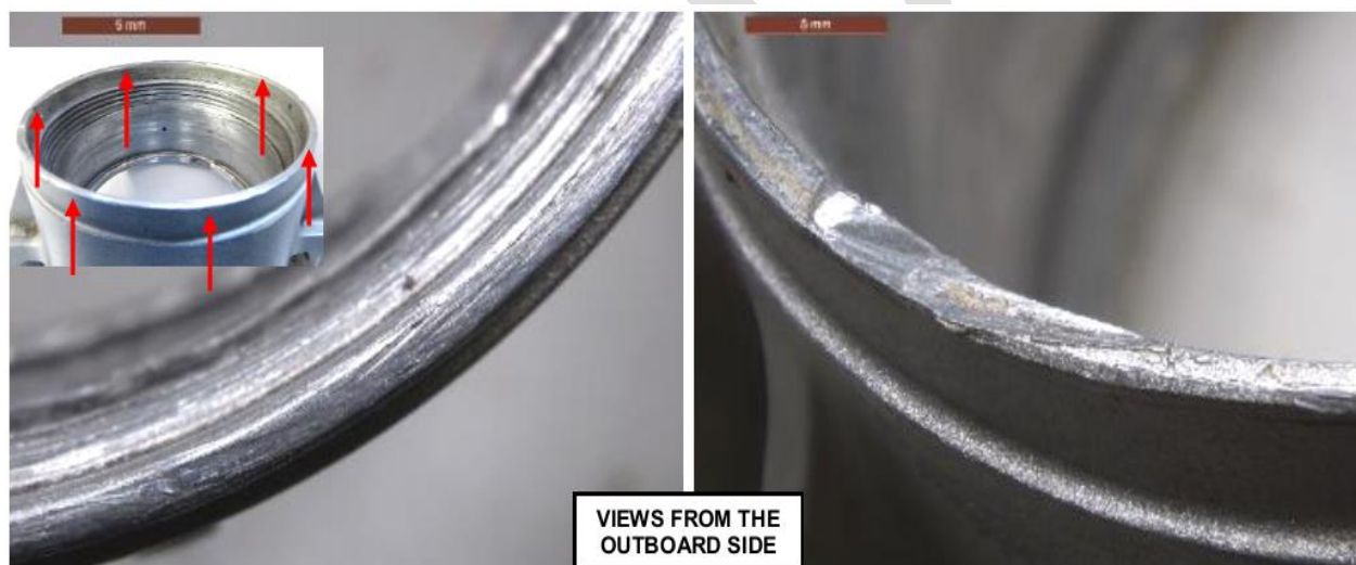
Figure 34 – Details of some crushed areas and inclined nicks visible on the outboard edge of the support bearing sleeve assembly (red arrows), due to the contact with the outboard locking nut after unscrewing.
