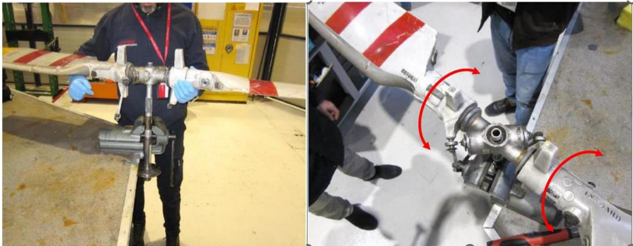
Figure 4 – Details of the test performed on the blades to verify the freedom of rotation around their longitudinal axis (red arrows). The hub was engaged on a test TR gear box output shaft.
