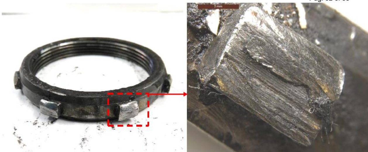
Figure 36 – Details of the crushed areas and inclined nicks visible on the relief elements of the inboard locking nut, due to the contact with the shoulder of the support bearing sleeve assembly mating with the inboard bearing.
