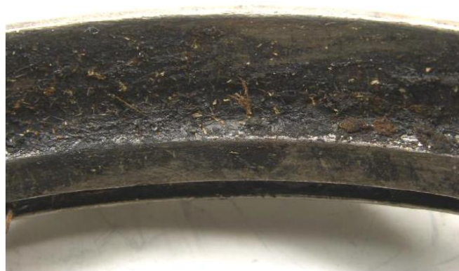
Figure 40 – Details of the duplex bearing outer rings with inner surface covered by soil-rich grease, as arrived in the laboratory.
