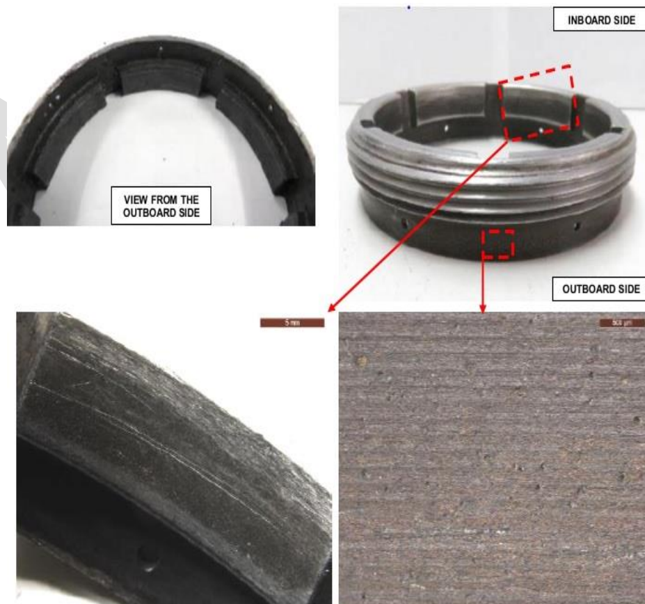
Figure 19 – Details of the outboard locking nut surfaces after cleaning. The nut is almost completely brown in color due to generalized oxidation.
