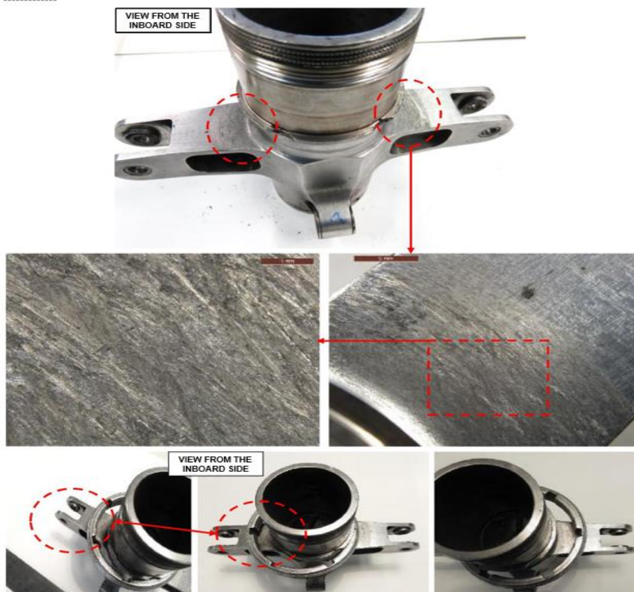
Figure 11 – Details of the worn areas (red circles) with rubbing morphology, observed on the pitch link arms of the slider assembly. The borders of the worn areas correspond to the circumferential edge of the locking nut when in contact to the slider central body.
