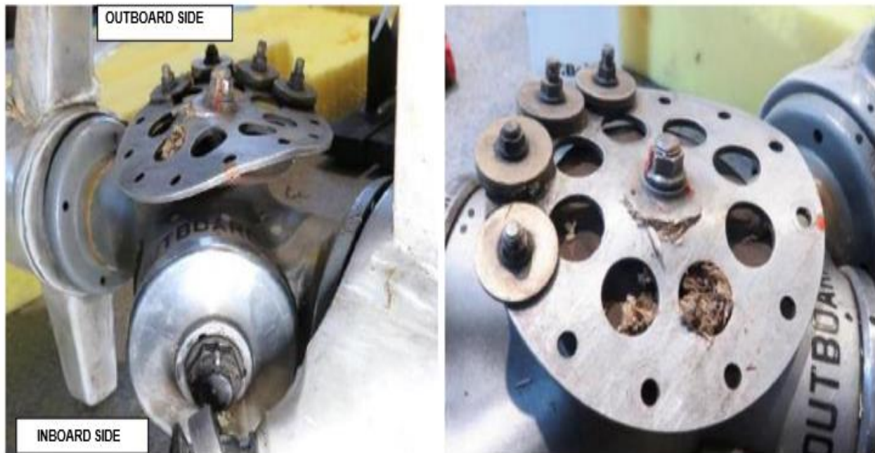
Figure 2 – Details of the deformed balancing flange and the absence of the washer to be installed mating to it (Fig. 1).
