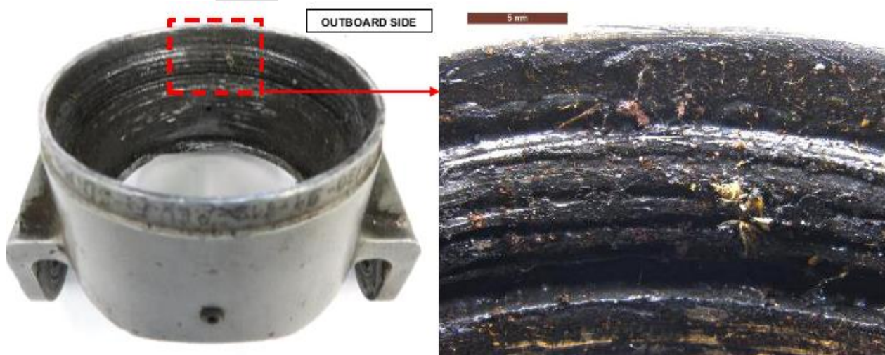
Figure 26 – Details of the support bearing sleeve assembly with inner surface covered by soil-rich duplex bearing grease and missing of the locking wires, as arrived in the laboratory.
