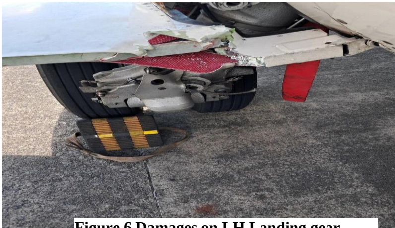
Figure 6. Damages on LH Landing gear
