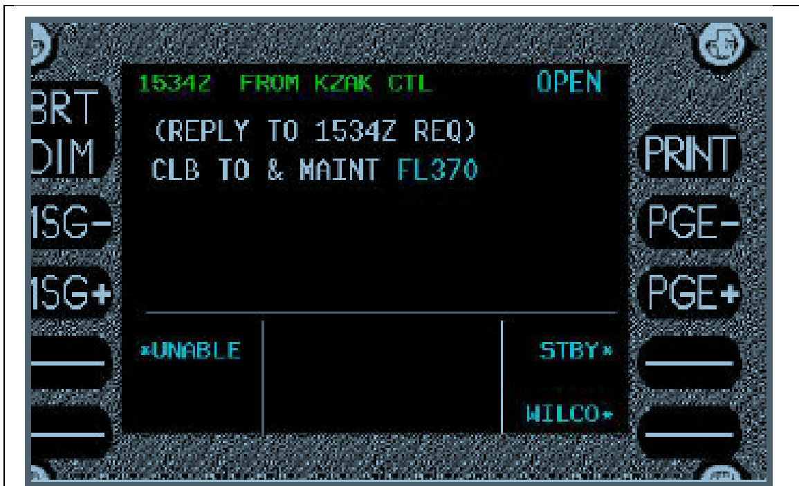
Fig 06B: Example of the reception of the ATC clearance to FL370 to a downlink request sent at 1534Z and linked with MRN.
