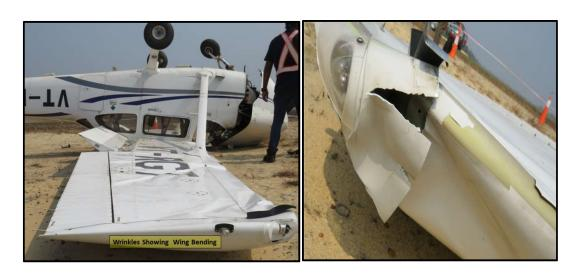
Figure 12: Damaged LH wing
