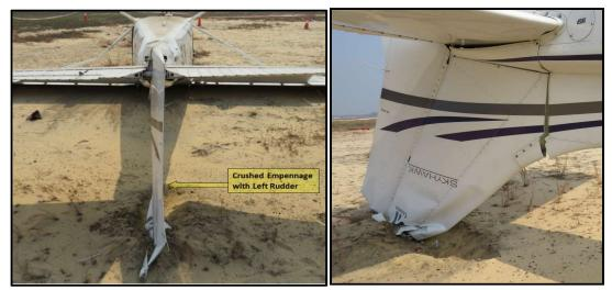
Figure 14: Damaged tail section
