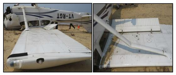
Figure 13 Damaged RH wing
