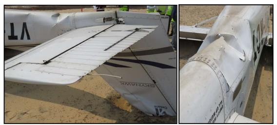
Figure 15: Damaged tail boom section
