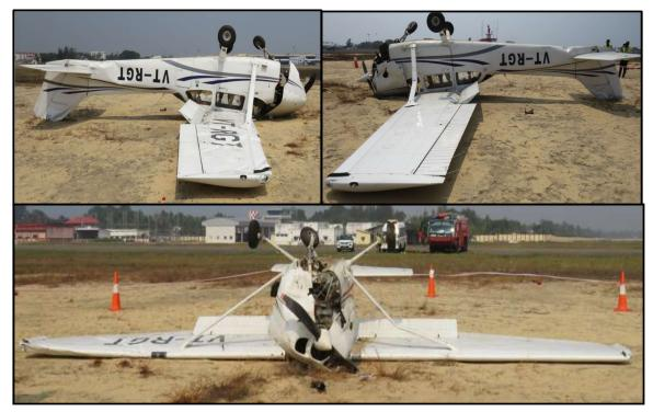
Figure 9: Aircraft Final Rest Position.
