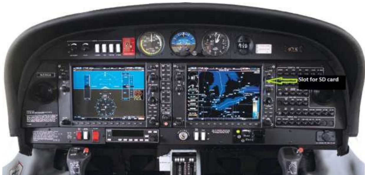
Figure 7: Garmin System (DA-40 Cockpit)
