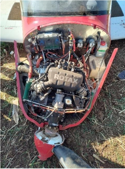
PIC3: NOSE SECTION & PROPELLER DAMAGED
