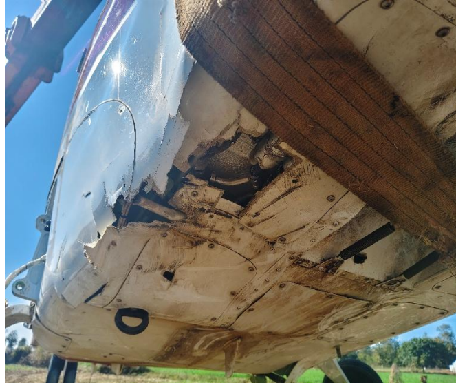
PIC4: FUSELAGE BOTTOM SKIN/STRUCTURE DAMAGED
